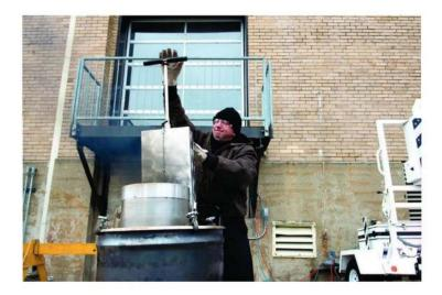
PHOTO: Basically a turbo-powered burn barrel, the wood-fueled Drug Terminator features a high-powered fan that creates a vortex of flame. Here, Sterling Deputy Police Chief jeff Mohr uses a tray and push rod to deliver a batch into the barrel. (Alex T. Paschal/apaschal@saukvalley.com)
